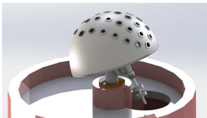
FIG. 1.—The Evryscope all-sky gigapixel-scale telescope currently under construction at UNC Chapel Hill. The system consists of 27 individual telescopes based on commodity hardware, encapsulated in a 1.8 m-diameter custom-molded dome which mimics the sky's hemisphere, and mounted on an off-the-shelf equatorial mount. See the electronic edition of the PASP for a color version of this figure.
