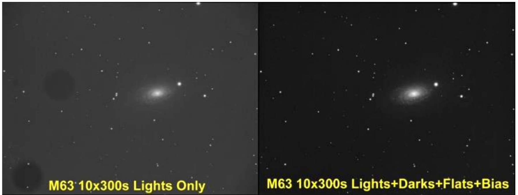
Figure 27. The galaxy Messier 63 with no corrections (left) and with the full Dark, Bias and Flat correction (right). Lights (Skys): 10x300s; Darks: 3x300s; Flats: 20x1.5s; Bias: 13x0.001s (Credit Jason Melquist)
