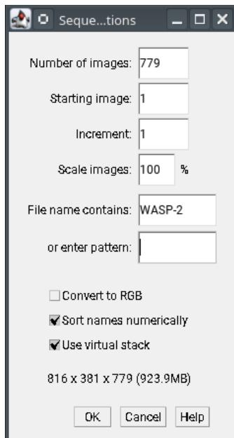
This tells you how many target images AIJ has found and will process. Verify that this is correct. In the above example, there are 779 science target image files (.fit files). If you want to make sure you are not unintentionally including any calibration images (like masterflat.fit), you can enter part of the target filename into the “file name contains” box. (Do not include an asterisk \* as a wildcard.)
