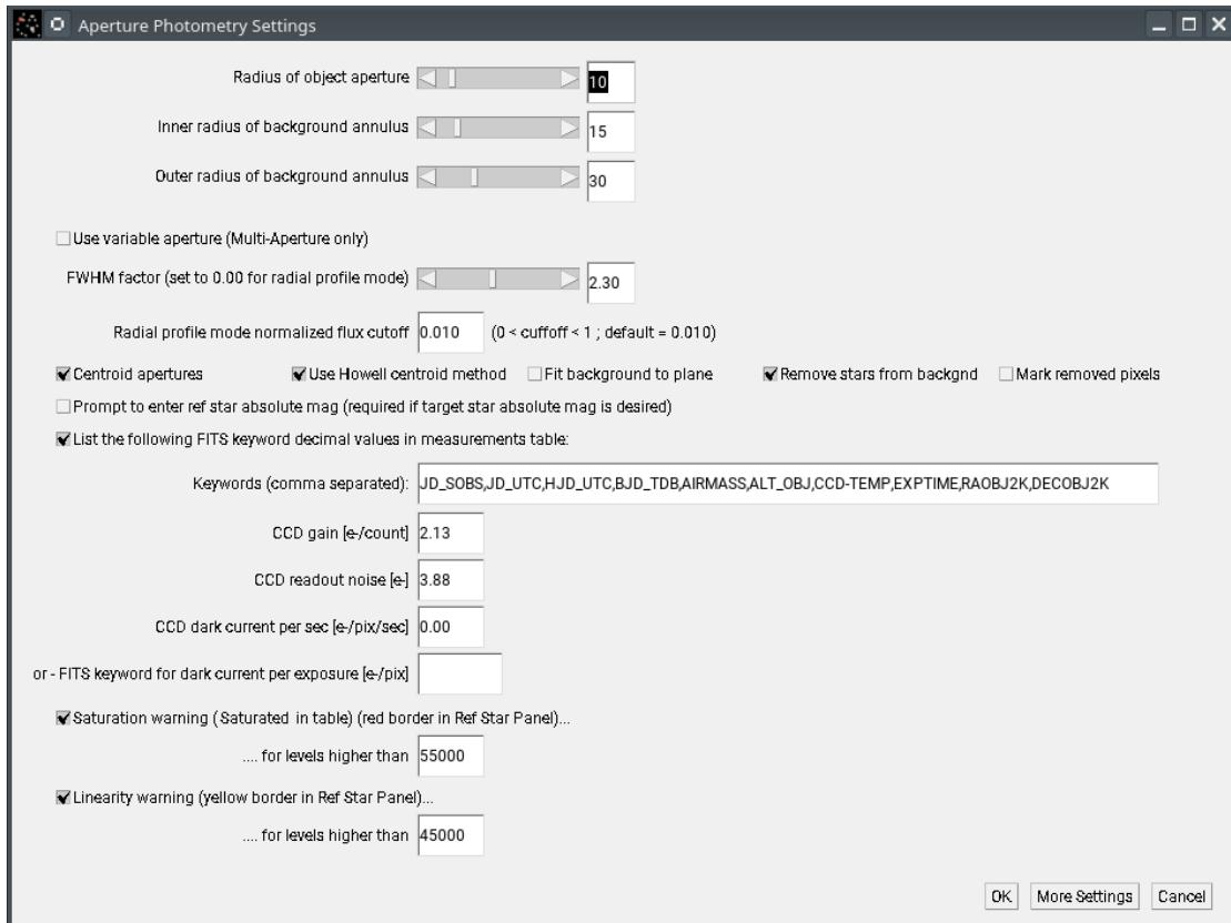
For MLO, the CCD has been tested to be linear up to 45,000 ADU. If you want to be cautious about the saturation you can choose number which are somewhat lower. These have no impact on the results, but a warning message will be recorded in the output file that the object may not be trustworthy if its peak exceeds these thresholds.
