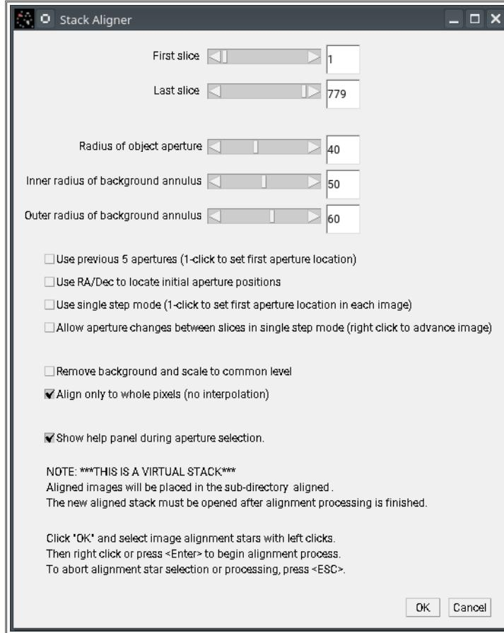
The first and last "slice" should correspond to the images in the sequence, and typically the first slice is 1 and the last slice is the number of science images to align. (This may be one less than the total number of images, since the first image won't be aligned - it is the reference image.)
