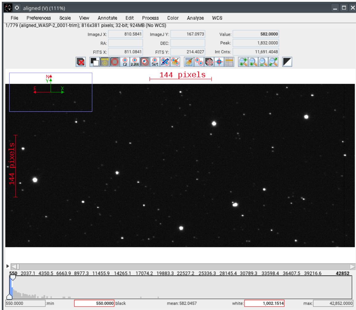
Verify that the correct number of images have been found by looking at the numbers just under the “File” tab in the upper left. In the above example, it says “1/779” (filename), meaning that this is the first of 779 images to be aligned.
